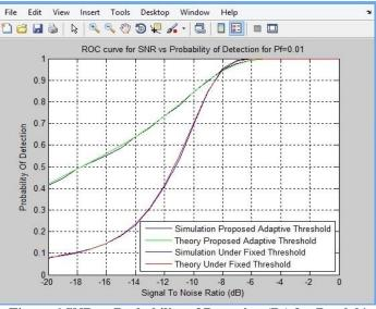
Figure.6 SNR vs Probability of Detection  $(P_d)$  for  $P_f = 0.01$
