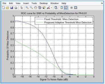
Figure.7 SNR vs Probability of Miss Detection (Pm) for Pf = 0.01
