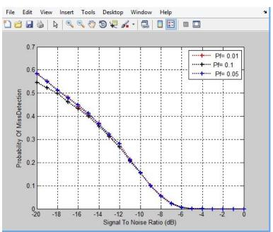
Figure.10 SNR vs Probability of Miss Detection  $(P_m)$  for  $P_f = 0.01, 0.1$  and 0.05
