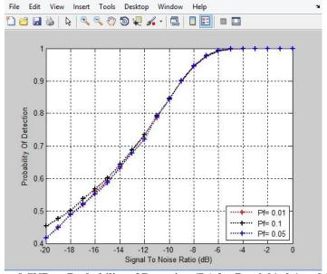
Figure.9 SNR vs Probability of Detection  $(P_d)$  for  $P_f = 0.01, 0.1$  and 0.05
